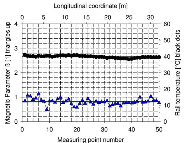
Fig. 4: Stress sensitive parameter and rail temperature, plotted vs. longitudinal coordinate.
