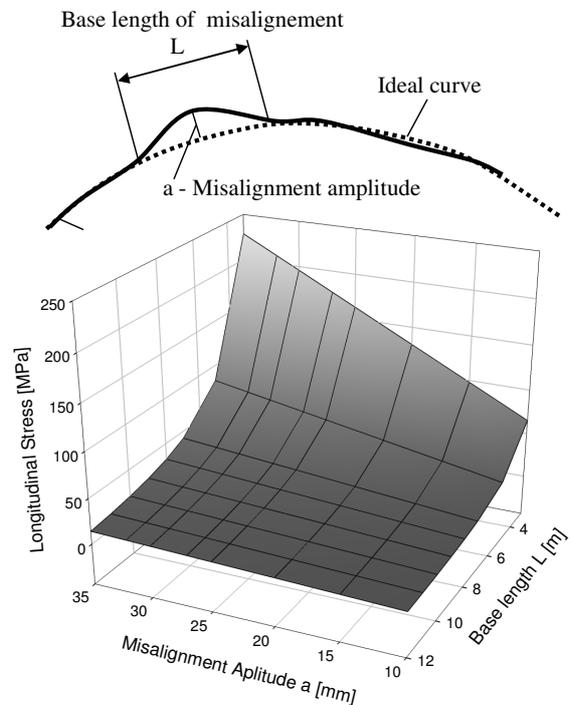
Fig. 11: Depiction of an alignment error situated in a curve and resulting bending stress
