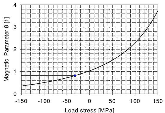
Fig. 5: Longitudinal load stress determined by means of the rail specific calibration curve.
