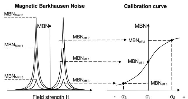
Fig.2: Calibration of MBN on load stress.
