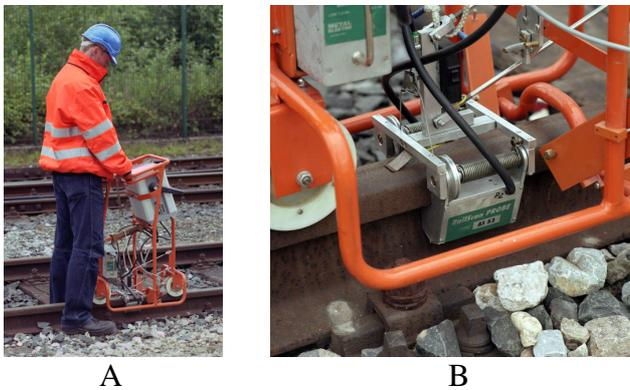
Fig. 3: Measuring device in use. A: Operator and device, B: Probe, coupled to the rail head.
