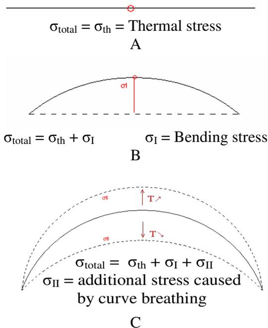
Fig. 8: A: Straight section without any misalignment- The total stress corresponds to the uniform longitudinal thermal stress, B: Curve without misalignment and high ballast resistance- The total stress consists of the thermal stress and the bending stress, C: Curve without misalignment and reduced ballast resistance- the total stress is supplemented by the bending stress caused by the curve breathing
