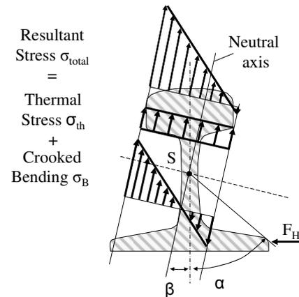
Fig. 9: Longitudinal stress and its crosssectional distribution in a bended cw-rail
