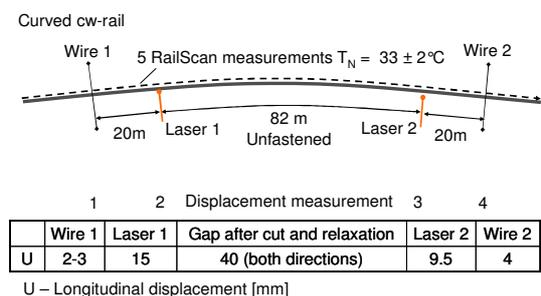
Fig. 7: Comparison measurement non-destructive – destructive and verification of anchor movement by displacement measurement
