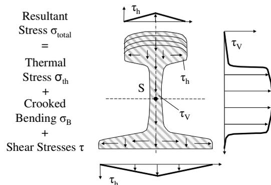
Fig. 10: Horizontal and vertical shear stresses caused by horizontal rail bending of the rail shown in fig. 8B and fig. 9
