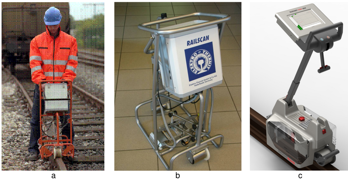
Fig. 2: Different RailScan and TRACKSAFE RELEASE device design generations. a: RailScan design from 2000 on, b: RailScan 2009/2010, c: TRACKSAFE RELEASE 2011 after full redesign
