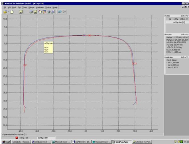
Figure 9: Ofot Line; Cross profile record (after weld installation)
