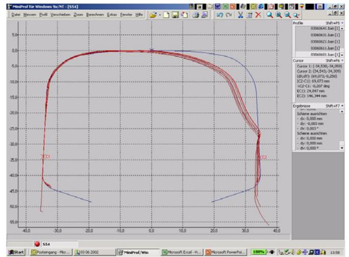
Figure 10: Ofot Line; HPW at 7,50 km; Cross profile record (after 22 months exposed to traffic)
