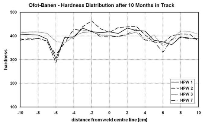
Figure 8: Ofot Line; In-track hardness measurement of HPW-welds (after 10 months exposed to traffic)
