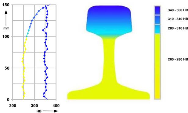
Figure 6: Hardness distribution within an HPW weld (vertical direction).
