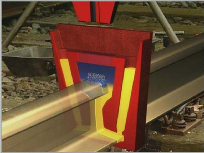
Figure 5: Principle of HPW – alloying elements are dissolved in weld head.
