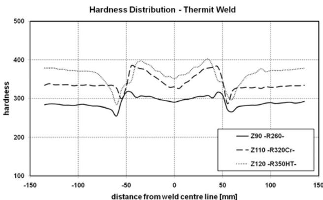
Figure 3: Hardness distribution in longitudinal direction of the weld (standard process).
