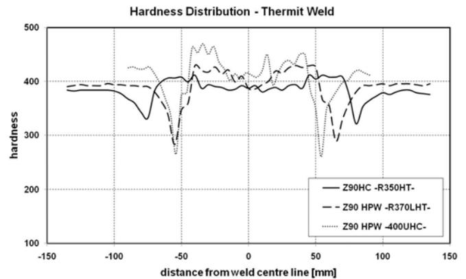
Figure 4: Hardness distribution in longitudinal direction of the weld (HC-procedure, HPW).
