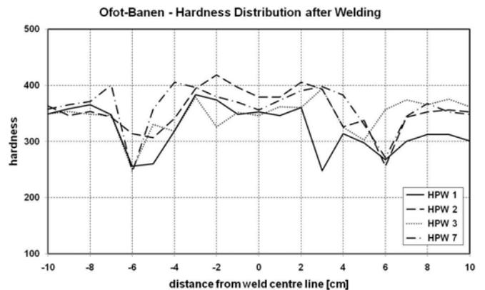
Figure 7: Ofot Line; In-track hardness measurement of HPW-welds (after installation)
